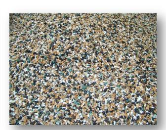
We start our molding process by purchasing 100% Post Consumer Recycled Plastics, we then add colorant and UV stabilizers to protect the finished products from the damaging rays of the sun. The end result is maintenance free products that will provide years of carefree service to the end user. Not only is it maintenance free but is Eco-friendly and will not harm the environment in any way. Sustainability at its finest can be found in all Polly Products.
